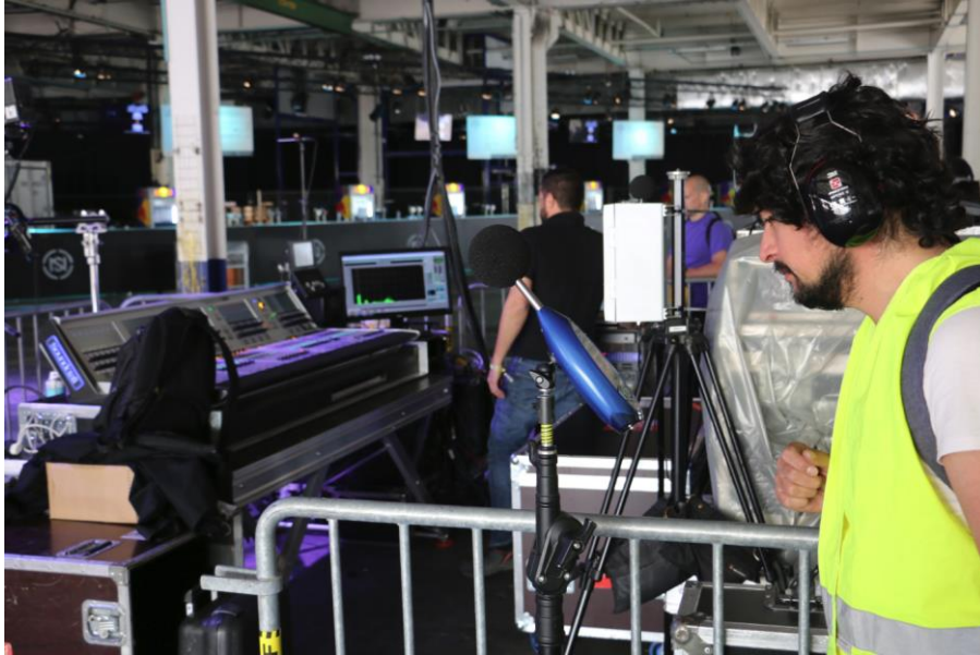
Figure 14: Complementary measurements (using pink noise) carried out during Nuits Sonores 2019 demonstrator. Reference point located at sound engineer’s console. Measurements carried out by Acoucity the day before the event.
