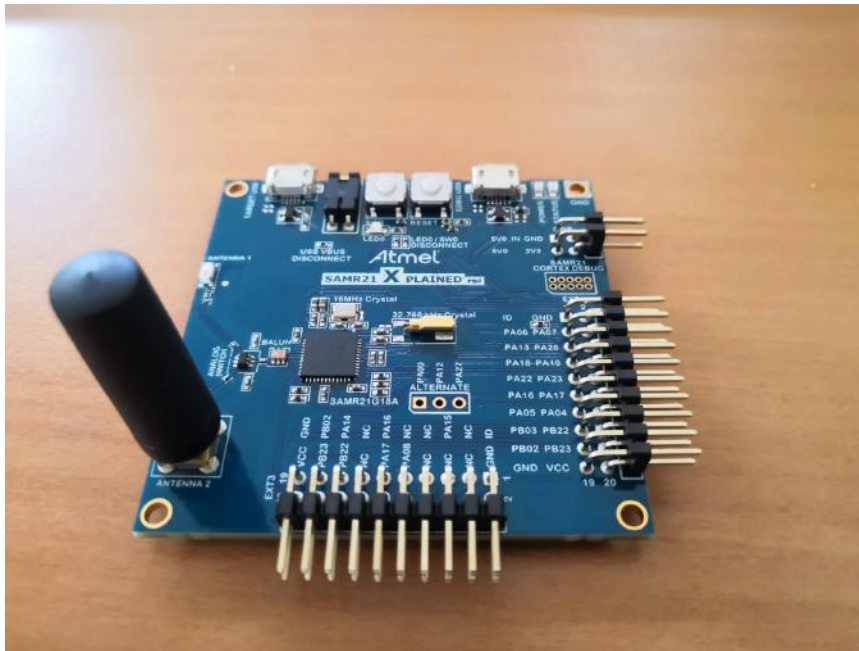
Figura 5.5: Microprocessore Atmel SAM R21 Xplained Pro
