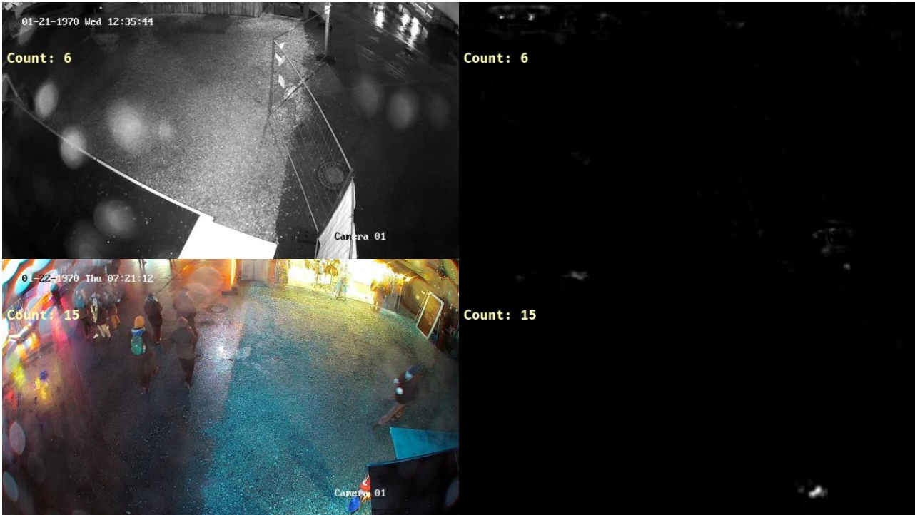
Figure 88 Example pictures showing results from the crowd algorithm. On the left the unprocessed, raw images from the camera stream and on the right the processed images, both show the crowd count
