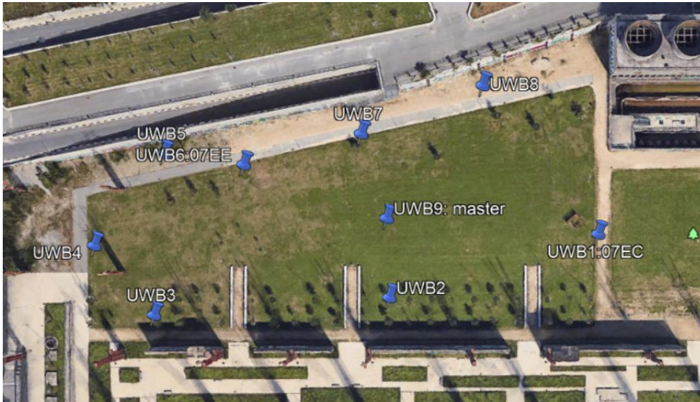
Figure 25 Positions of 9 UWB anchors for staff wristbands deployed in KFF18
