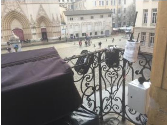
Figure 104 Point A IoT SLM on the YCM balcony, in front of Place Saint-Jean
