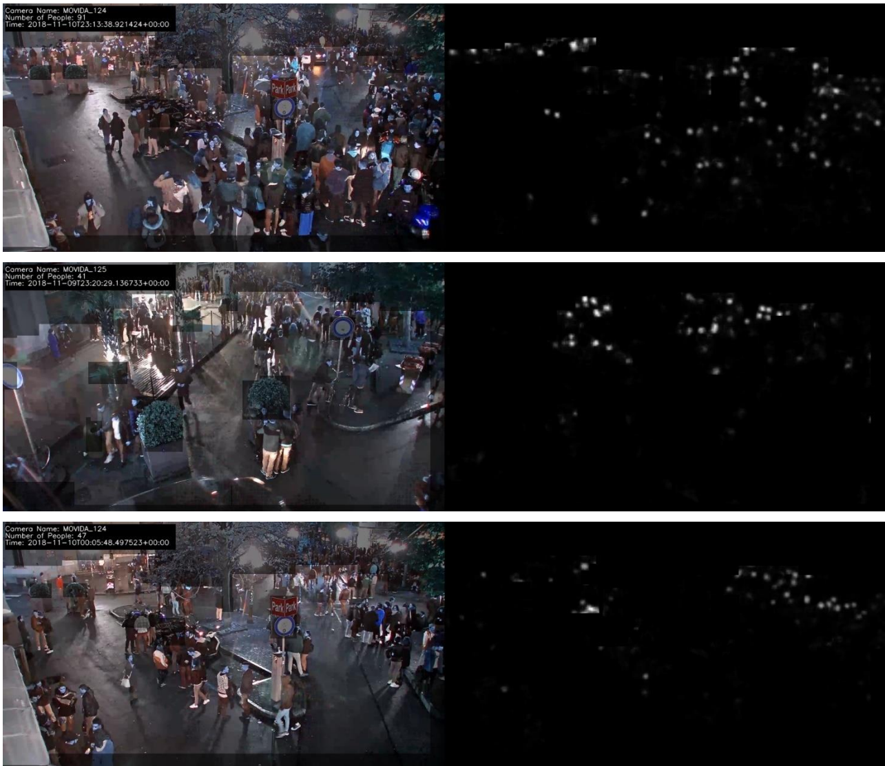
Figure 81 Three examples of crowd density: (left) the original frames captured from the camera with the mask, camera info, time and total count overlaid. (right) the density maps produced by the algorithm, where white areas represent people
