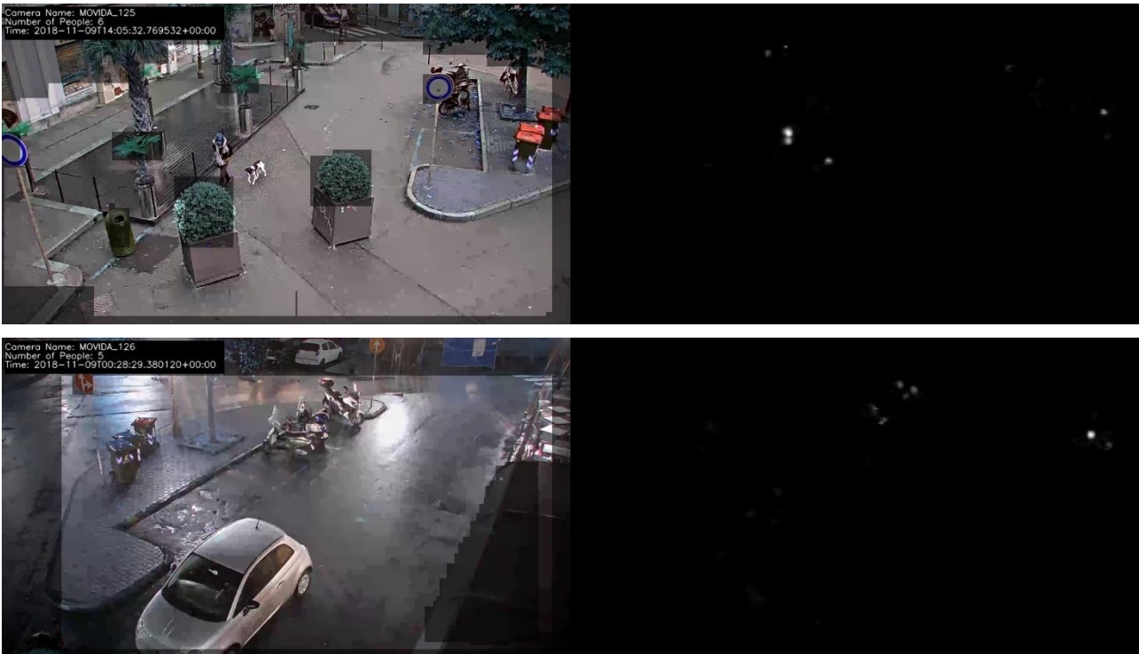
Figure 83 Examples of mis reads where objects such as cars or bikes produce false results
