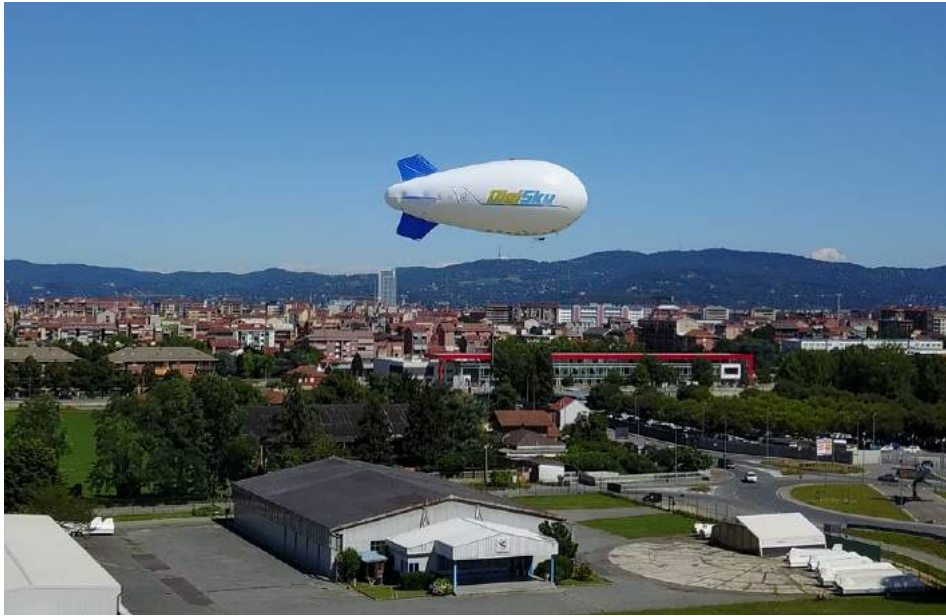
Figure 63: The DigiSky blimp prototype floating over the Aeritalia Airport, Turin (Ground Operators not visible in the picture are controlling the Blimp altitude through cables connected to Ground)
