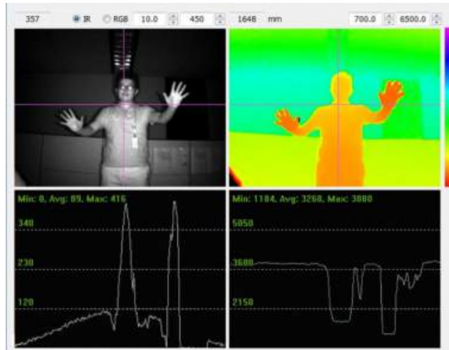
Figure 54: (a) Infrared illumination image (b) Depth image (c) Illumination variation across the image for the selected horizontal line (d) Depth variation across the image for the selected horizontal line
