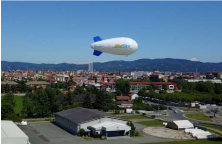
Figure 43: The DigiSky blimp prototype floating over the Aeritalia Airport, Turin (Ground Operators not visible in the picture are controlling the Blimp altitude through cables connected to Ground)
