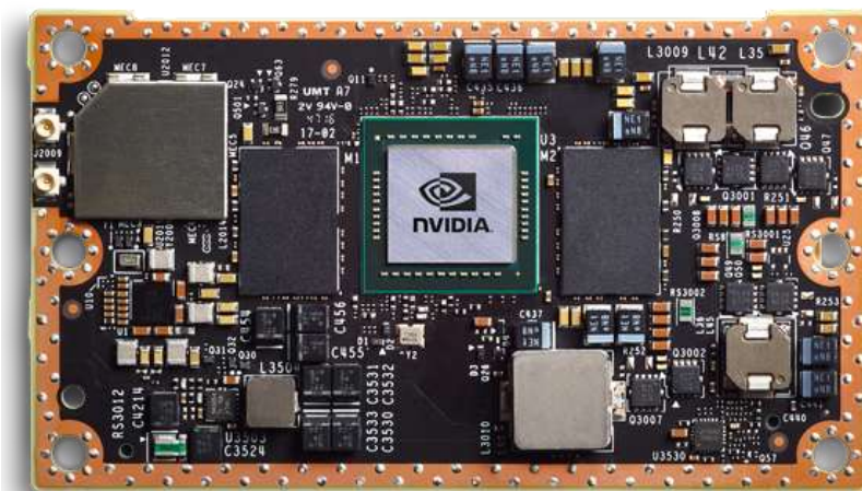
Figure 37: nVIDIA TX2 embedded GPU single-board-computer (SBC)
