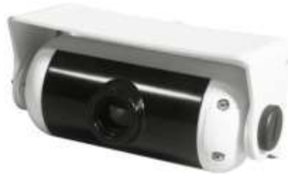
Figure 32: Time-of-flight depth camera with embedded video analytics
